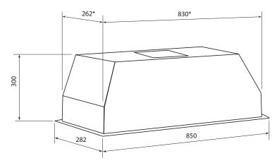
\* allow 5mm clearance for installation
